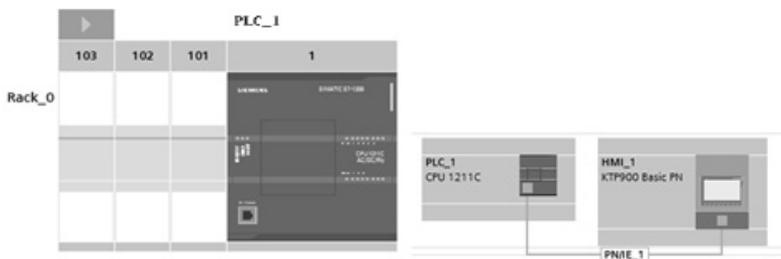
Figure. 3. PLC and HMI simulation in Tia Portal
