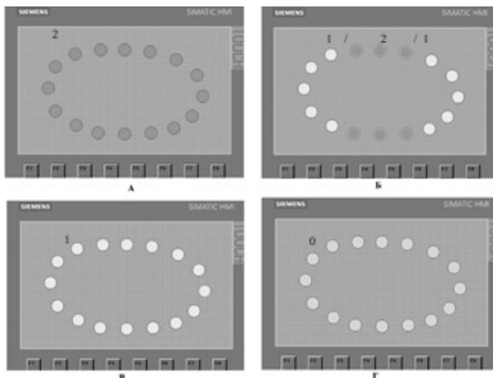
Fig. 4. Stadium lighting simulation modes a) powerful lighting mode b) normal lighting mode c) energy saving lighting mode d) lighting off
